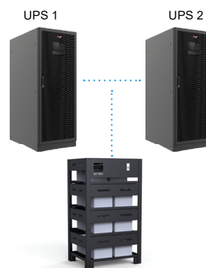
Common battery bank
